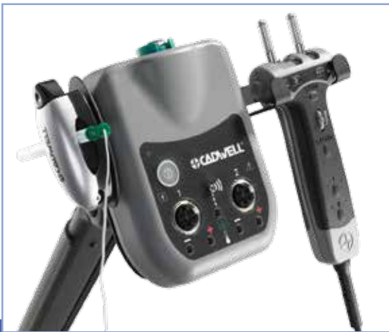
Amplifier bracket with 2 channel amplifier, stimulator and needle holder
