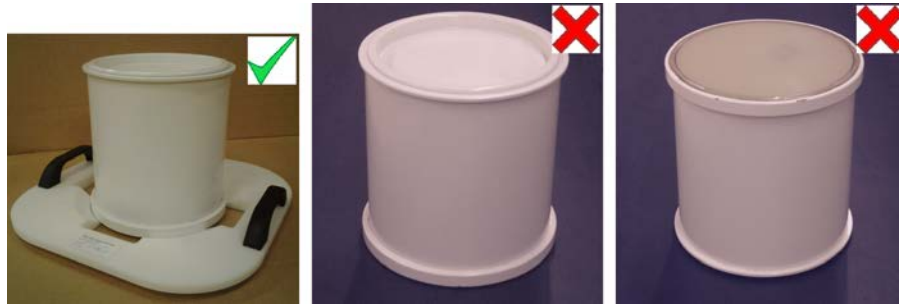
Fig. 115: Store the QA phantom on the QA Phantom Plate with the membrane facing down.
