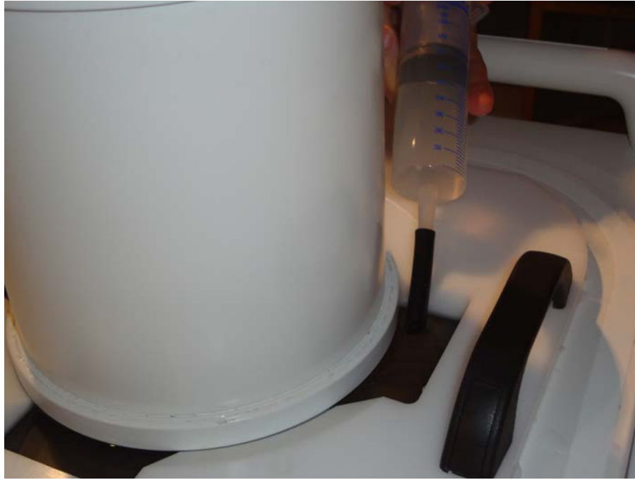
Fig. 108: Fill any remaining air pockets under the phantom with degassed water.
