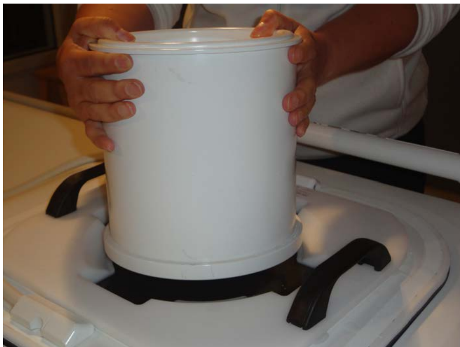
Fig. 107: Place one edge of the QA phantom on the phantom plate. Gently lower the QA phantom onto the phantom plate.
