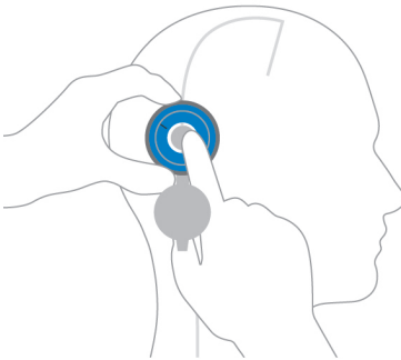
Fig. 17: Adjustment using the M.blue plus Adjustment Ring
