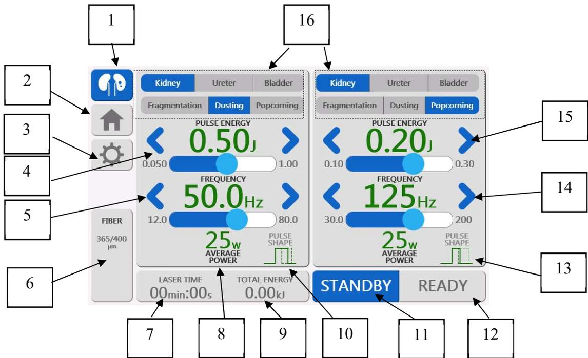
Figure 15. Screen for setting the laser radiation parameters for the STONE preset mode
