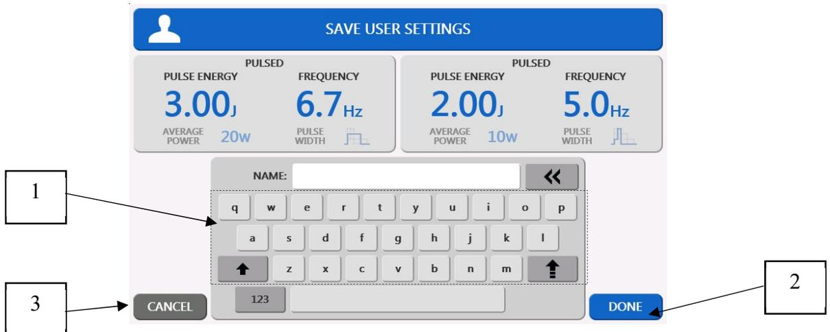
Figure 21. Screen for saving the laser radiation parameters
