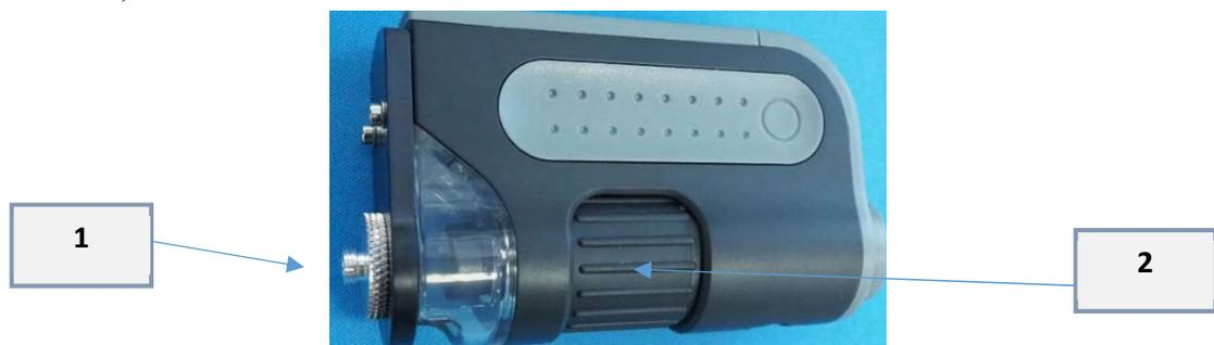
Fig. 11. Microscope for inspecting the fiber end in the connector
