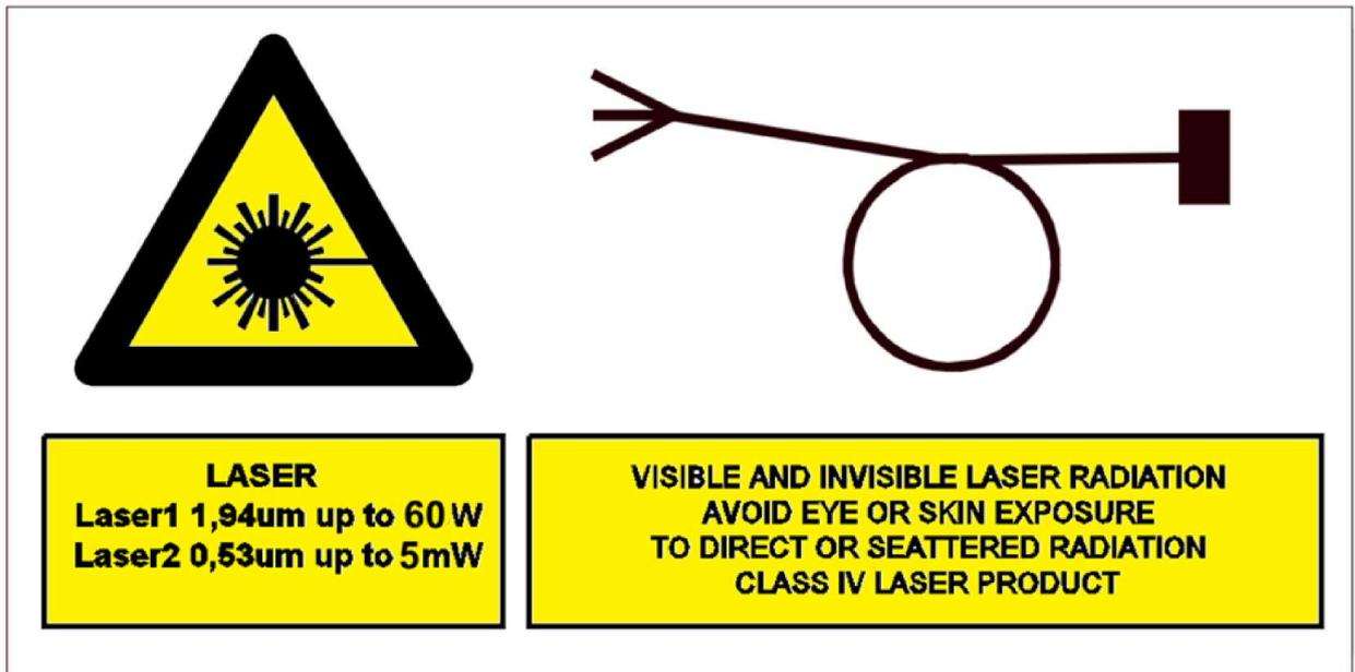
Figure 1b. Laser hazard signs for Urolase SP+
