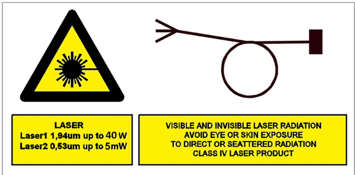
Figure 1c. Laser hazard signs for Urolase SP
