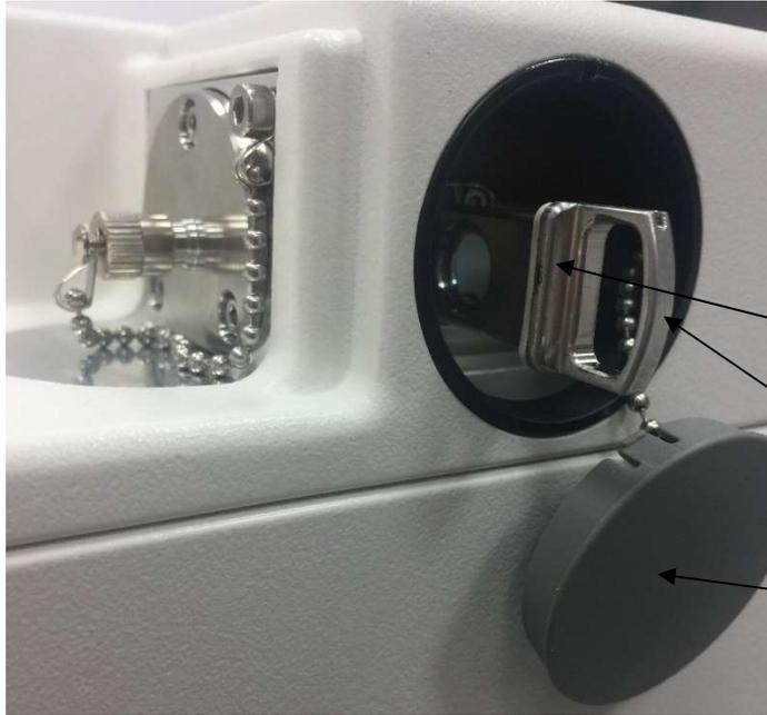
Insert new protective window (2) until it stops (ledge (1) on the protective window should be located on the left when installing onto the Device) and close the cover (3). After installing a new protective window with the Device turned on, the error on the screen should disappear.
