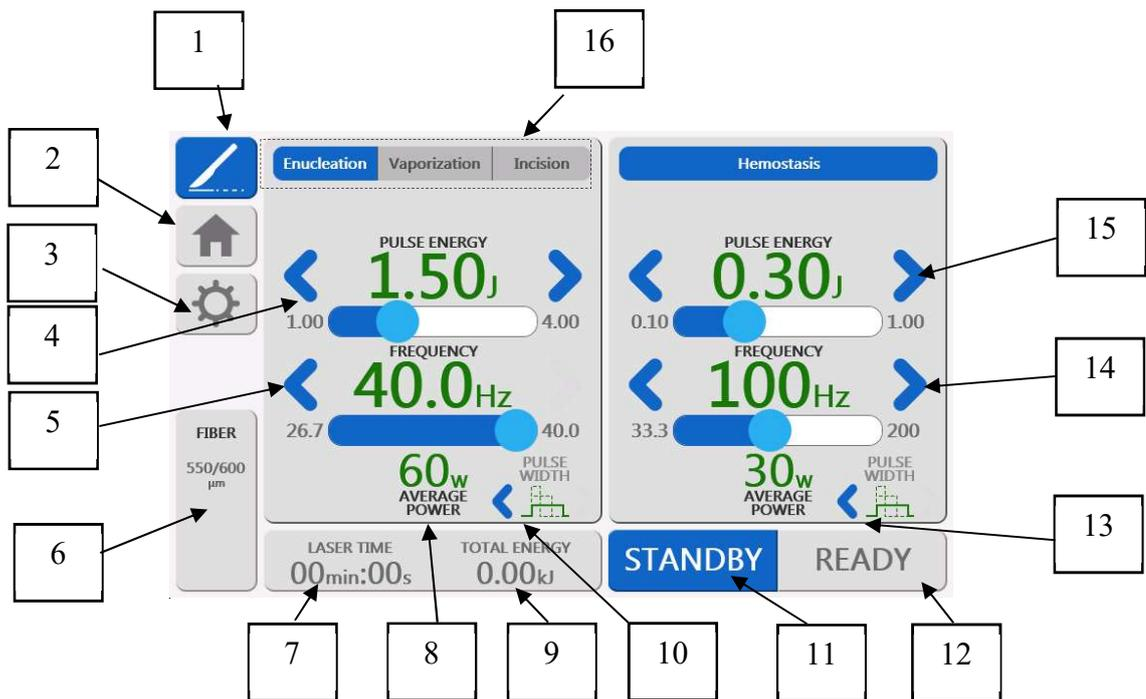
Figure 19. Screen for setting laser radiation parameters for the SOFT TISSUES preset mode
