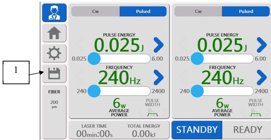
Figure 20. Screen for setting laser radiation parameters in the EXPERT preset mode
