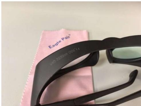
Fig. 12.4 – Marking: OD5+ optical density goggles, protection in the wavelength range from 980 to 2500 nm.
