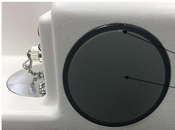
The protective window is located behind the cover (1). To access the protective window, open the cover (1). To do this, place a pointed item (such as a flat screwdriver, tweezers, etc.) in the hole (2).
